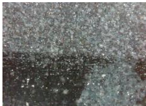
h) uzorak korodiran u otopini \text{Na}_2\text{S}_2\text{O}_5 , prijelaz
